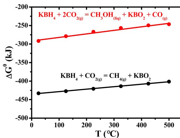
**Fig. 8 – Calculated standard free energy changes as a function of temperature for 2 possible routes of  $\text{CO}_2$  uptake by  $\text{KBH}_4$  using the data source [52].**
