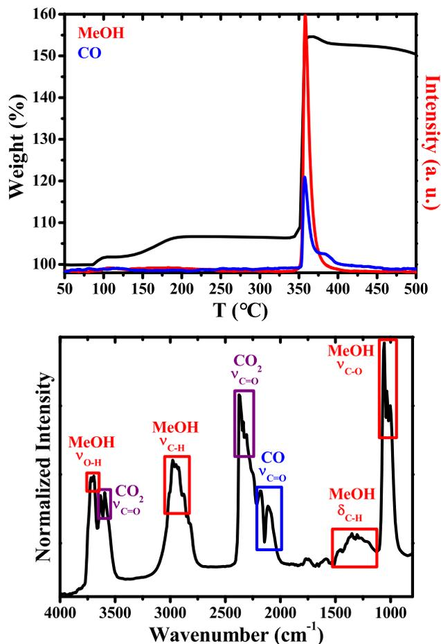
Fig. 7 – TGA-FTIR of the solid–gas reaction of  $KBH_4$  with  $CO_2$  (top) and the FTIR spectrum of the gas products formed at 360 °C (bottom), the temperature is plotted for the reference curve.
