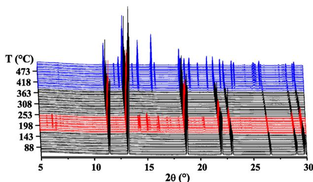
**Fig. 9** – Variable temperature in situ synchrotron X-ray powder diffraction ( $\lambda = 0.775045 \text{ \AA}$ ) of  $\text{KBH}_4$  under the  $\text{CO}_2$  atmosphere (30 bar).
