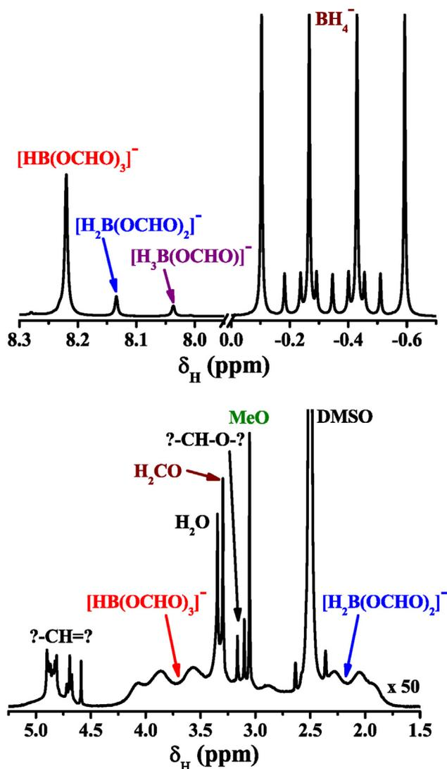
Fig. 3 – The  $^1\text{H}$  NMR spectrum of the product obtained after ball milling. The cut out part of the spectrum is shown in the bottom graph.
