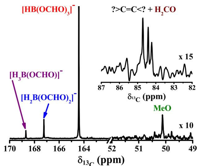
Fig. 2 – The  $^{13}\text{C}\{^1\text{H}\}$  NMR spectrum of the product obtained after ball milling.
