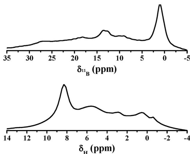
**Fig. 10** –  $^1\text{H}$  (bottom) and  $^{11}\text{B}\{^1\text{H}\}$  (top) solid-state NMR spectra of the sample obtained in autoclave synthesis by keeping  $\text{KBH}_4$  at  $116 \text{ }^\circ\text{C}$  under 32 bar of  $\text{CO}_2$  for 140 min; the corresponding diffraction data are shown in Fig. S4 in Supplementary data.
