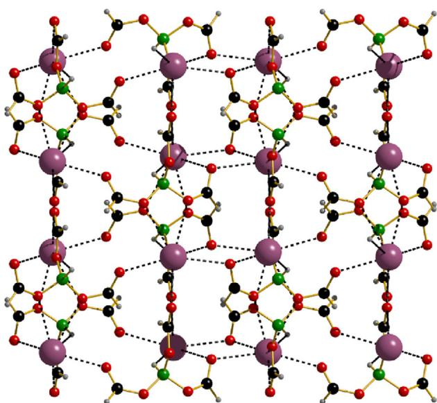
Fig. 5 – Crystal packing of  $\{K[HB(OCHO)_3]\}_n$  along the  $c$  axis. Color code: B = green, C = black, H = gray, K = purple, O = red. (For interpretation of the references to color in this figure legend, the reader is referred to the web version of this article.)
