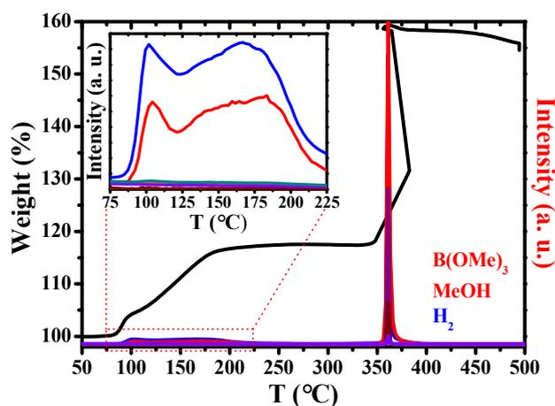
Fig. 6 – TGA-MS of the solid–gas reaction of  $KBH_4$  with  $CO_2$ .
