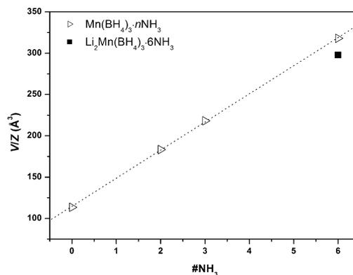
**Figure 7.** Unit cell volumes ( $V$ ) at RT divided by the number of formula units ( $Z$ ) plotted as a function of the number of ammonia molecules in the formula unit,  $Mn(BH_4)_2 \cdot nNH_3$  ( $n = 0, 2, 3, 6$ ). The unit cell volume of  $Li_2Mn(BH_4)_4 \cdot 6NH_3$  subtracted the volume of two formula units of  $LiBH_4$  (data from Ref. [47]) is shown as a black square.
