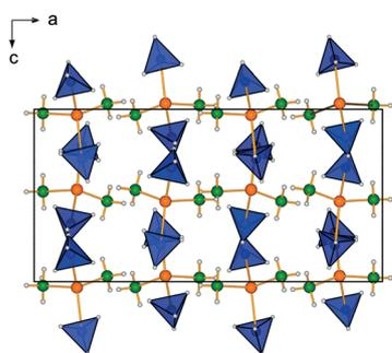
**Figure 5.** The crystal structure of  $Mn(BH_4)_2 \cdot 2NH_3$ .  $Mn^{2+}$  (orange) is coordinated by two  $NH_3$  molecules (N green) and two  $BH_4^-$  complexes (blue tetrahedron), forming neutral molecular complexes,  $[Mn(NH_3)_2(BH_4)_2]$ . Hydrogen atoms are light gray.
