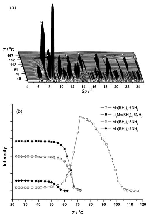
**Figure 9.** (a) In situ SR-PXD of  $\text{Mn}(\text{BH}_4)_2 \cdot 6\text{NH}_3$ - $\text{Mn}(\text{BH}_4)_2$  (3:3, s6) heated from RT to 200 °C ( $5^\circ\text{C min}^{-1}$ ,  $p(\text{Ar}) = 1 \text{ bar}$ ,  $\lambda = 0.823056 \text{ \AA}$ ). (b) Integration of selected reflections plotted as a function of the temperature. Symbols:
