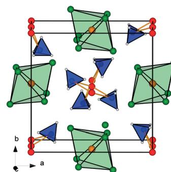
**Figure 6.** The crystal structures of  $Li_2Mn(BH_4)_4 \cdot 6NH_3$ . Manganese,  $Mn^{2+}$  (orange), is octahedrally coordinated by six nitrogen atoms (N green) in  $NH_3$  molecules forming  $[Mn(NH_3)_6]^{2+}$  complexes. Lithium,  $Li^+$  (red), is coordinated by four  $BH_4^-$  complexes (blue tetrahedra) forming a  $[Li_2(BH_4)_4]_n^{2-}$  polymer along the [001] direction. Hydrogen atoms are light gray in  $BH_4^-$ , while hydrogen atoms in  $NH_3$  are now shown for simplicity.
