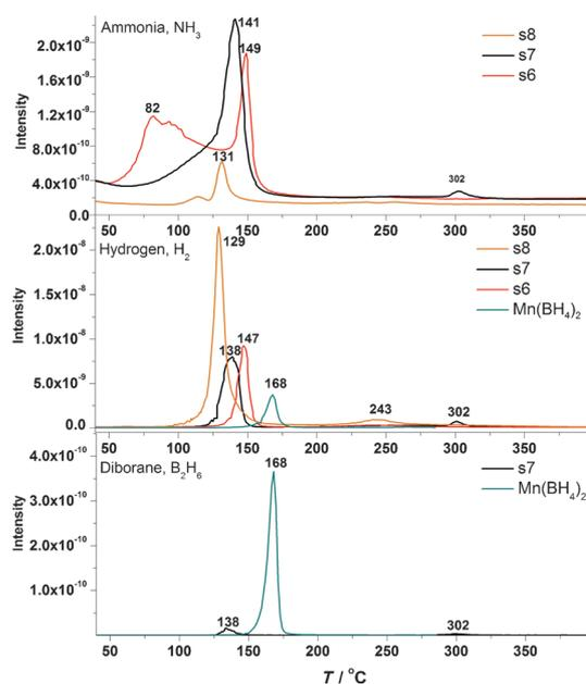
Figure 12. Mass spectrometer signals for NH<sub>3</sub> (upper), H<sub>2</sub> (middle) and B<sub>2</sub>H<sub>6</sub> (lower) of Mn(BH<sub>4</sub>)<sub>2</sub> and Mn(BH<sub>4</sub>)<sub>2</sub>·6NH<sub>3</sub>-Mn(BH<sub>4</sub>)<sub>2</sub> (3:3, s6), (2:4, s7) and (1:5, s8) heated from RT to 400 °C (5 °C min<sup>-1</sup>).
