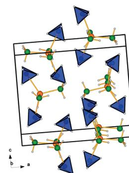
**Figure 4.** The crystal structure of  $\text{Mn}(\text{BH}_4)_2 \cdot 3\text{NH}_3$ . Manganese ions,  $\text{Mn}^{2+}$  (orange), coordinates to three  $\text{NH}_3$  (N green) groups and two  $\text{BH}_4^-$  (blue tetrahedron) forming neutral molecular complexes in the solid state,  $[\text{Mn}(\text{NH}_3)_3(\text{BH}_4)_2]$ . Hydrogen atoms are light gray.
