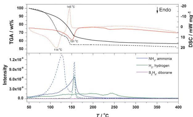
**Figure 10.** Thermogravimetric analysis and differential scanning calorimetry coupled with a mass spectrometer measured for  $\text{Mg}(\text{BH}_4)_2 \cdot 6\text{NH}_3$  (s1, solid line) and  $\text{Mn}(\text{BH}_4)_2 \cdot 6\text{NH}_3$  (s2, dashed line) heated from RT to 400 °C ( $5^\circ\text{C min}^{-1}$ ). The upper diagram shows the TGA curves (black lines) and DSC-profiles (red lines), while the lower diagram shows the corresponding MS-signals.
