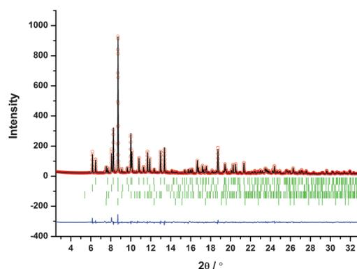
**Figure 1.** Rietveld refinement of SR-PXD data for  $\text{Mn}(\text{BH}_4)_2 \cdot 6\text{NH}_3$ - $\text{Mn}(\text{BH}_4)_2$  (3:3, s6) measured at RT,  $\lambda = 0.823065$  Å. “Tic marks”  $\text{Mn}(\text{BH}_4)_2 \cdot 3\text{NH}_3$  (top),  $\text{Li}_2\text{Mn}(\text{BH}_4)_4 \cdot 6\text{NH}_3$ ,  $\text{Mn}(\text{BH}_4)_2 \cdot 2\text{NH}_3$  and  $\text{Mn}(\text{BH}_4)_2 \cdot 6\text{NH}_3$ .
