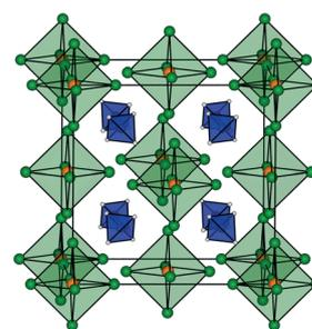
**Figure 3.** The crystal structure of  $\text{Mn}(\text{BH}_4)_2 \cdot 6\text{NH}_3$ .  $\text{Mn}^{2+}$  (orange) is octahedrally coordinated by six N-atoms (N green) in  $\text{NH}_3$  molecules forming the complex  $[\text{Mn}(\text{NH}_3)_6]^{2+}$ , while  $\text{BH}_4^-$  (blue tetrahedron) acts as counter ions in the crystalline solid. Hydrogen atoms in  $\text{BH}_4^-$  are light gray, while hydrogen atoms in  $\text{NH}_3$  are now shown for simplicity.
