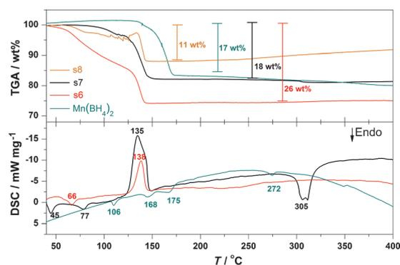
Figure 11. TGA/DSC for Mn(BH<sub>4</sub>)<sub>2</sub> and Mn(BH<sub>4</sub>)<sub>2</sub>·6NH<sub>3</sub>-Mn(BH<sub>4</sub>)<sub>2</sub> (3:3, s6), (2:4, s7) and (1:5, s8) heated from RT to 400 °C (5 °C min<sup>-1</sup>). DSC data for s8 are not shown.
