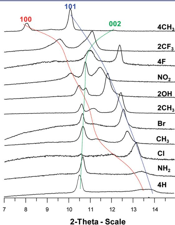
**Figure 2.** XRPD ( $\lambda_{\text{Cu}} \approx 1.79 \text{ \AA}$ ) of the dried forms of the various functionalized MIL-88B samples. Dotted lines for the three first Miller indices have been added for easier tracking.
