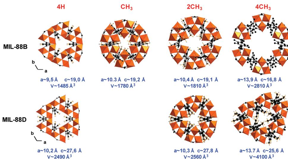
**Figure 4.** View along the *c* axis of one pore of the dried MIL-88B, MIL-88(CH<sub>3</sub>), MIL-88B(2CH<sub>3</sub>) and MIL-88B(4CH<sub>3</sub>), MIL-88D, MIL-88D(2CH<sub>3</sub>), and MIL-88D(4CH<sub>3</sub>) solids. Metal polyhedra, carbon atoms, and hydrogen atoms are in orange, black, and gray, respectively. The corresponding cell parameters are provided for a better understanding.
