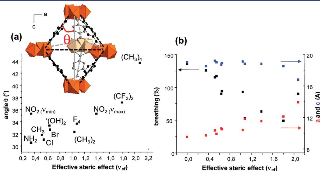
**Figure 3.** Variation of (a) the  $\theta$  angle of the bipyramid characteristic of the MIL-88 structure in the dried form and (b) the swelling amplitude and the unit cell parameters  $a$ ,  $c$  versus the effective steric parameter of the functional group. Insert (top left): definition of the angle  $\theta$  (hydrogen atoms are omitted for clarity; metal polyhedral and carbons are in orange and black, respectively).
