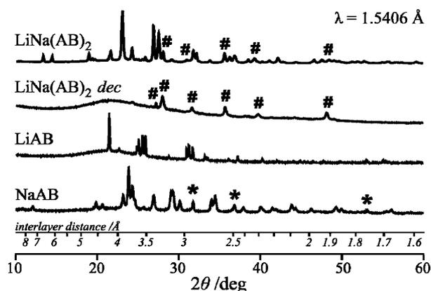
**Fig. 1** Comparison of X-ray powder diffraction data (CuK radiation) for  $\text{LiNa}(\text{AB})_2$  (top) and single-cation amidoboranes of lithium and sodium (bottom). Reflections from NaH (\*) and WC (#) are marked.
