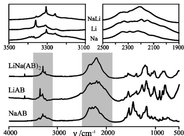
**Fig. 4** Comparison of the FTIR spectra of  $\text{LiNa}(\text{AB})_2$  and of the constituent single-cation amidoboranes of lithium and sodium. The ranges marked in grey are shown magnified at the top.
