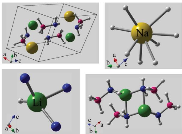
**Fig. 3** The crystal structure of  $\text{NaLi}(\text{AB})_2$ : (left top) crystallographic unit cell; (right top) the first coordination sphere of  $\text{Na}^+$  at  $<2.6$  Å; (left bottom) the first coordination sphere of  $\text{Li}^+$  at  $<2.3$  Å; (right bottom) projection emphasizing the presence of dimeric  $[\text{Li}(\text{AB})_2]^-$  anions. H white, B red, N blue, Li green, Na yellow. Positions of light H atoms are tentative and should be taken with care.
