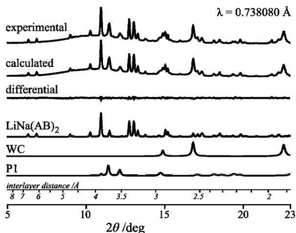
**Fig. 2** Rietveld decomposition of the diffractogram of  $\text{NaLi}(\text{AB})_2$  (synchrotron radiation) showing all phases present in the sample:  $\text{NaLi}(\text{AB})_2$ , WC, and unknown *P1* phase (see text).
