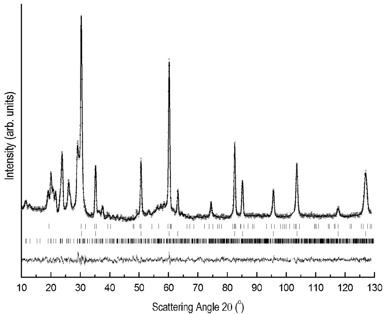
**Fig. S1:** Powder neutron diffraction pattern for  $\text{LiZn}_2(^{11}\text{BD}_4)_5$  (sample A) measured at 295 K showing observed (circles), calculated (upper line) and difference (bottom line) plots. The position of the Bragg reflections are shown as tic marks for  $\text{LiZn}_2(^{11}\text{BD}_4)_5$  (lower),  $\text{LiCl}$  (middle), and  $\text{ZnCl}_2$  (upper) ( $\lambda = 1.55499 \text{ \AA}$ ).
